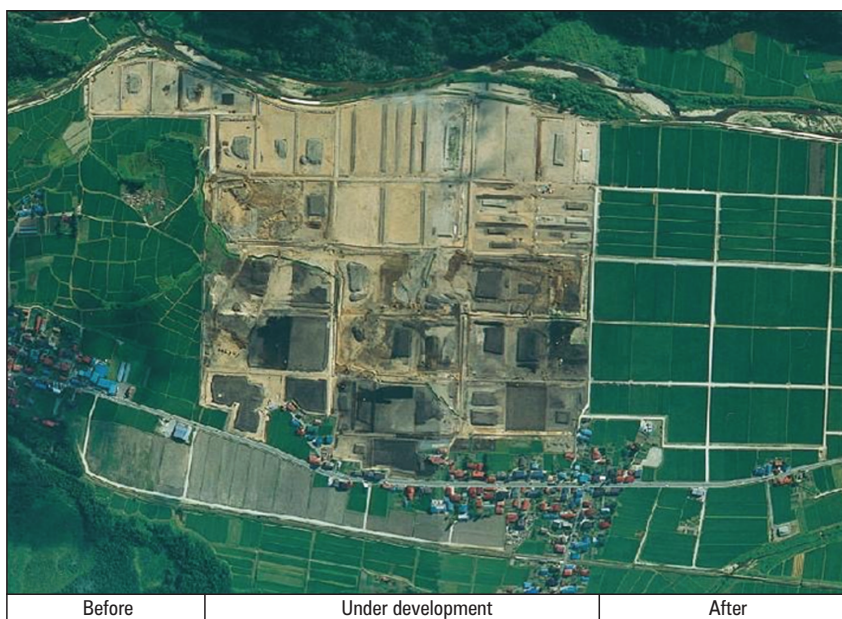
Fig. 1. Change in landscape through a land consolidation project in Mogami town, Yamagata prefecture. This shows how the project transformed irregular and smaller farm plots (left) into larger and regular farm plots (right) with access to farm roads and irrigation and drainage canals
